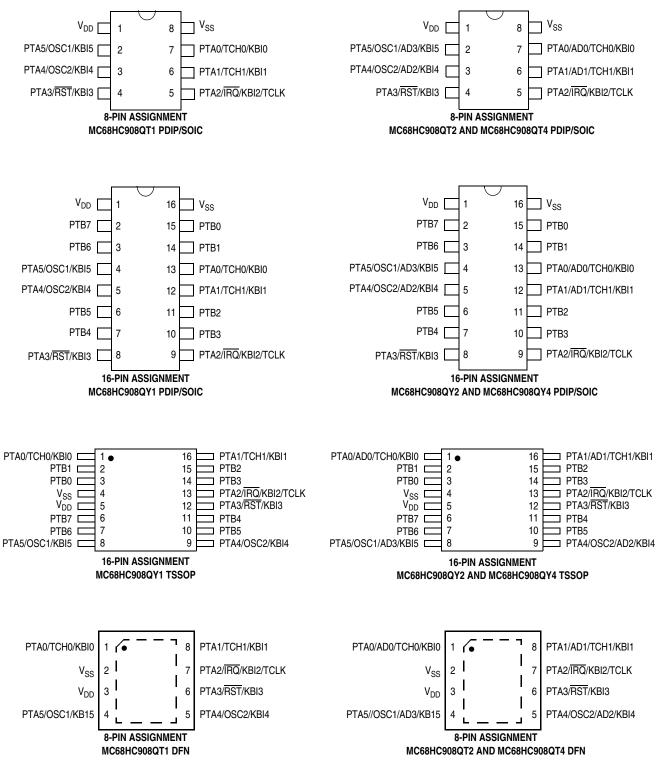
Figure 1-2. MCU Pin Assignments
