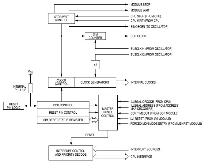
Figure 13-1. SIM Block Diagram
