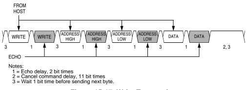
Figure 15-17. Write Transaction
