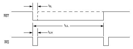
Figure 16-7.  $\overline{RST}$  and  $\overline{IRQ}$  Timing
