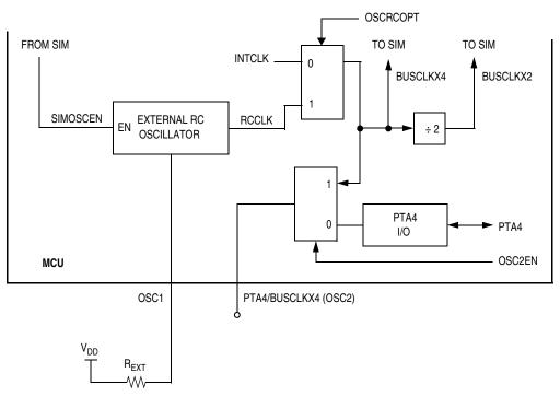
See Section 16. Electrical Specifications for component value requirements.
