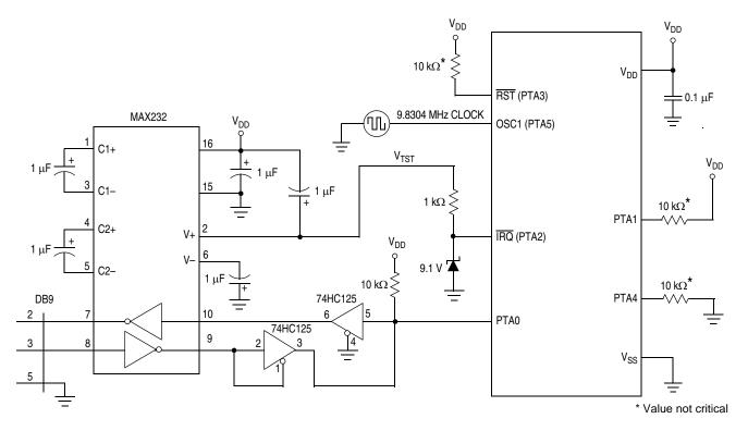
Figure 15-11. Monitor Mode Circuit (External Clock, with High Voltage)
