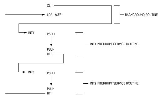
Figure 13-11. Interrupt Recognition Example
