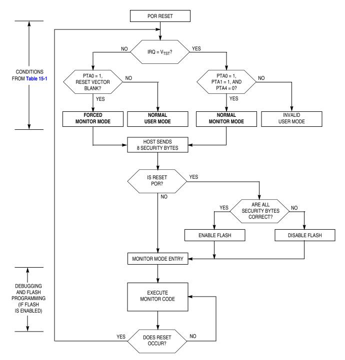
Figure 15-10. Simplified Monitor Mode Entry Flowchart
