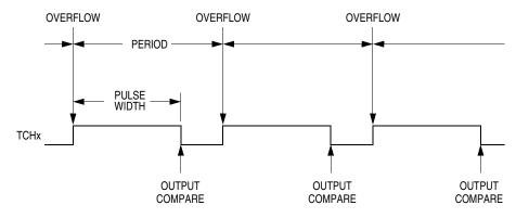
Figure 14-4. PWM Period and Pulse Width
