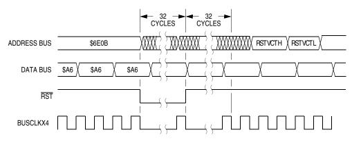
Figure 13-17. Wait Recovery from Internal Reset
