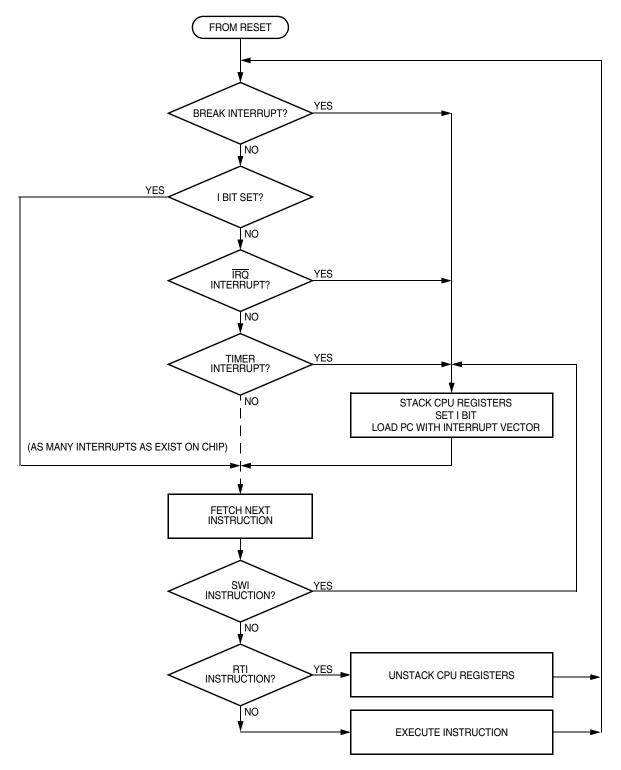
Figure 13-8. Interrupt Processing
