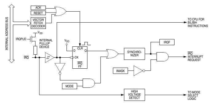
Figure 8-2. IRQ Module Block Diagram
