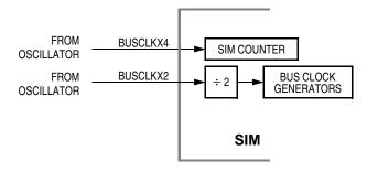
Figure 13-3. SIM Clock Signals
