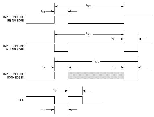
Figure 16-11. Timer Input Timing
