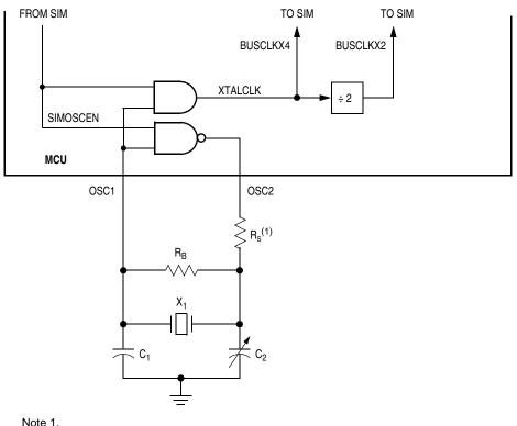
R<sub>s</sub> can be zero (shorted) when used with higher-frequency crystals. Refer to manufacturer's data. See Section 16. Electrical Specifications for component value recommendations.
