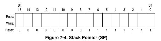
**NOTE:** The location of the stack is arbitrary and may be relocated anywhere in random-access memory (RAM). Moving the SP out of page 0 (\$0000 to \$00FF) frees direct address (page 0) space. For correct operation, the stack pointer must point only to RAM locations.
