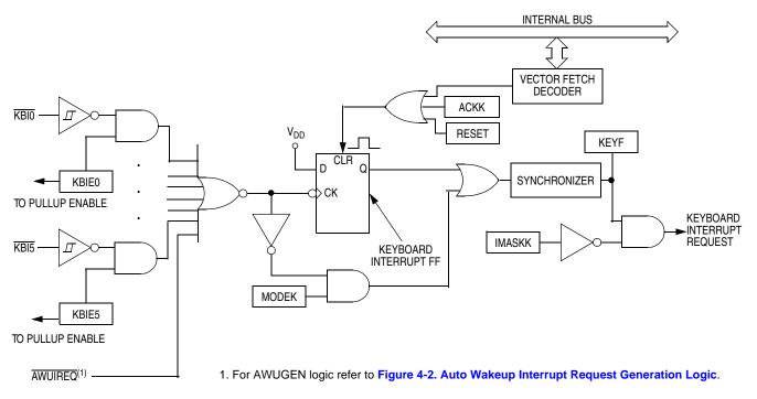
Figure 9-3. Keyboard Interrupt Block Diagram
