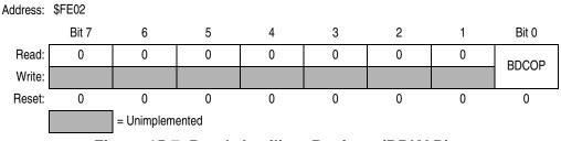
Figure 15-7. Break Auxiliary Register (BRKAR)
