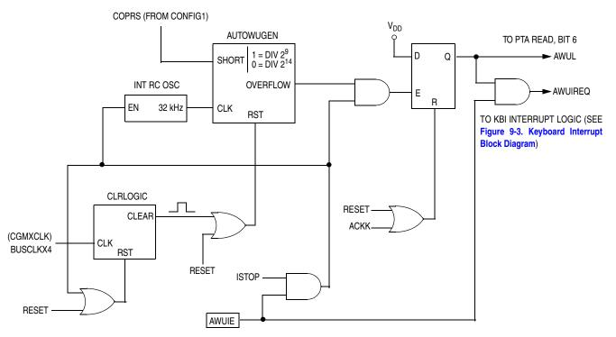
Figure 4-2. Auto Wakeup Interrupt Request Generation Logic
