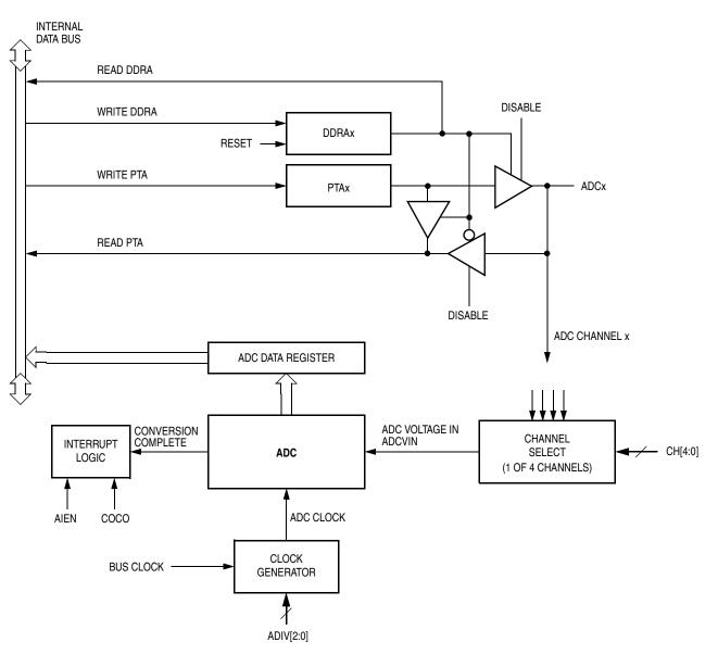
Figure 3-3 shows a block diagram of the ADC.
