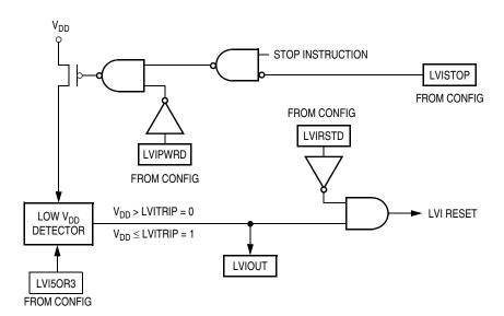
Figure 10-1. LVI Module Block Diagram
