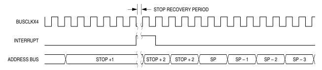
Figure 13-19. Stop Mode Recovery from Interrupt
