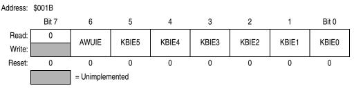
Figure 9-5. Keyboard Interrupt Enable Register (KBIER)
